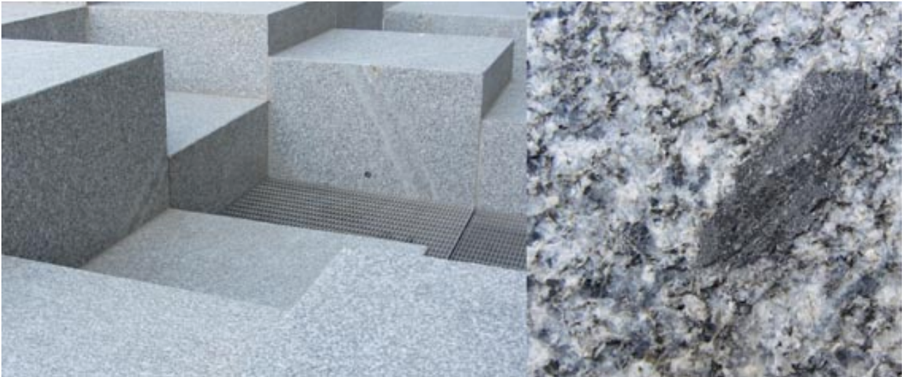
The Giant's Causeway seating blocks and a close up of Azul Extremadura granite showing a small xenolith of black schist. The field of view (FOV) is 5 cm.
