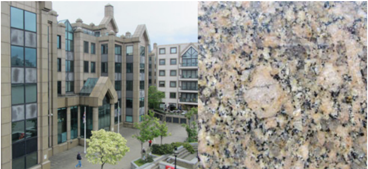
Left: Millennium Bridge House, Right: Golden Carioca granite, field of view is 10 cm.
