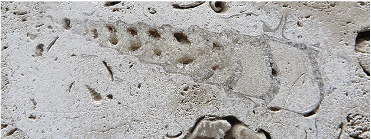
Above: Portland Roach used for cladding on the Economist Plaza entrance of Ryder Street. Below: detail of a Portland Screw infilled with secondary calcite spar.
