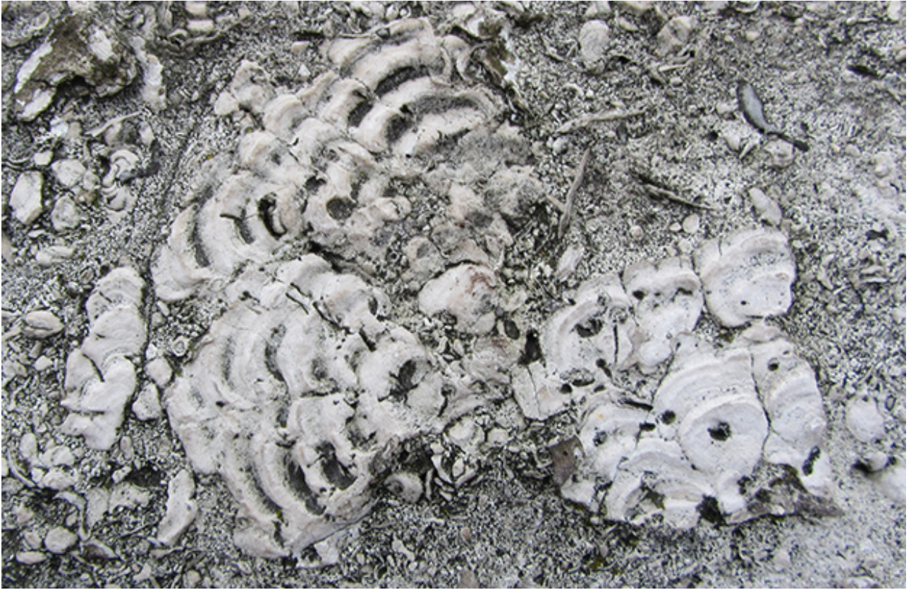
Above: Solenopora weathering out on the parapet of Waterloo Bridge . FOV 5 cm.
