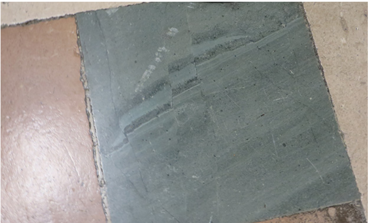
Figure 3. A paving stone of Ordovician, Cumbrian Green Slate. This stone shows small-scale faulting of layers of bedded volcanic ash.
