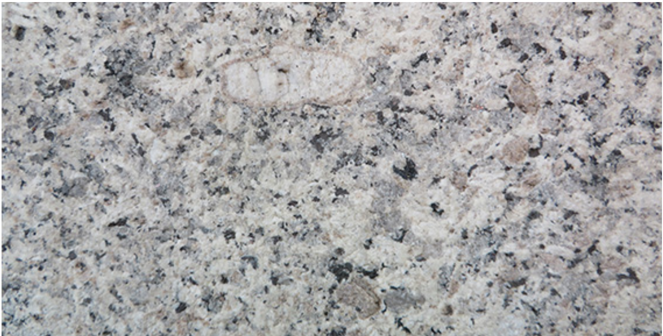
The granite used on the Submarine Memorial (see below); note the pink feldspar and the white feldspar megacrysts with a pink rim (top centre). Field of view is ~ 20 cm.
