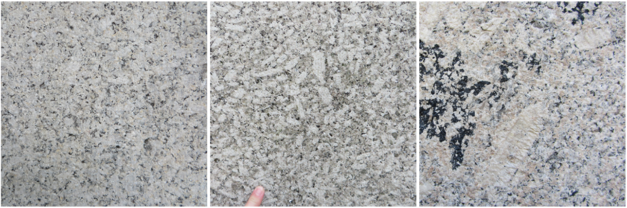
Left: Non-porphyritic granite; Middle: Small megacrystic granite; Right: Large megacrystic granite. All images are at the same scale.
