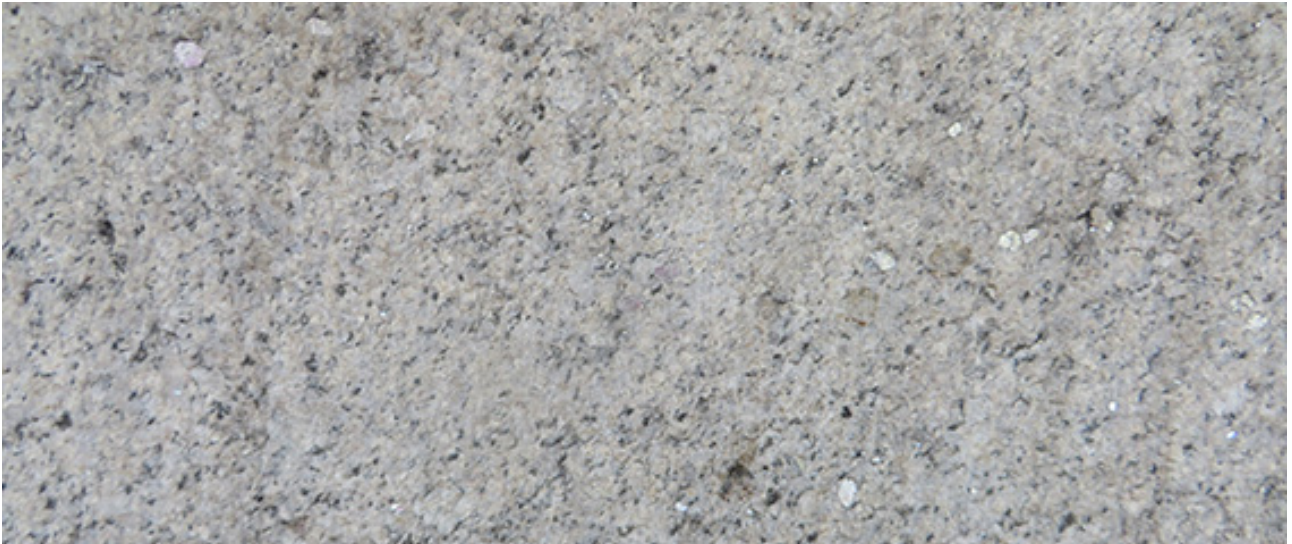
'Muscovite Granite' Possibly from Killiney, Ireland. Note the prominent flakes of silver muscovite, ~ 3-5 mm diameter. Field of view ~ 25 cm.
