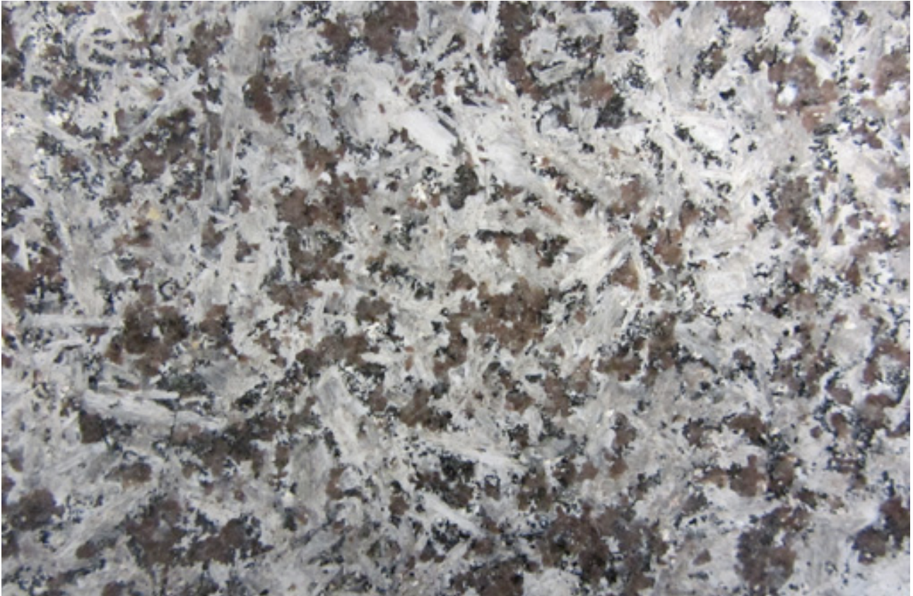
Polished slab of foyaitite (UCL Earth Sciences), Field of view is ~ 15 cm. The rock is composed of white alkali feldspar, brown nepheline, black pyroxene and mica.
